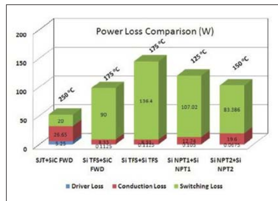
Figure 6: Overall loss comparison of Sjt and silicon IGBTs at their maximum operating temperature. The results are given for a 100 kHz switching frequency
