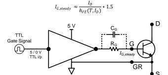
Figure 21: TTL Gate Drive Schematic
