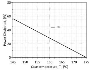
Figure 16: Power Derating Curve
