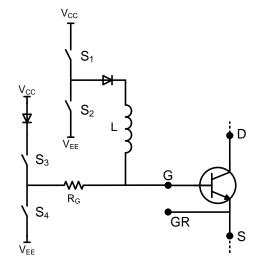
Figure 26: Simplified Inductive Pulsed Drive Topology
