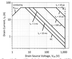
Figure 18: Forward Bias Safe Operating Area at  $T_c$ = 25  $^{\circ}$ C
