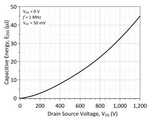
Figure 10: Energy Stored in Output Capacitance
