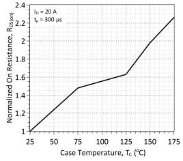
Figure 6: On-Resistance vs. Temperature
