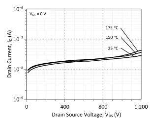
Figure 8: Typical Blocking Characteristics
