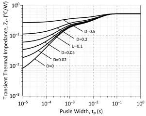
Figure 20: Transient Thermal Impedance
