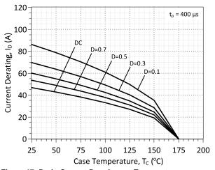
Figure 17: Drain Current Derating vs. Temperature
