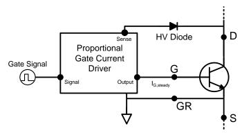
Figure 27: Simplified Voltage Controlled Proportional Driver
