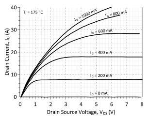
Figure 3: Typical Output Characteristics at 175 °C
