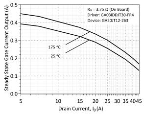
Figure 24: Typical steady state gate current supplied by the GA03IDDJT30-FR4 board for the GA20JT12-263 with the on board resistance of 3.75  $\Omega\,$
