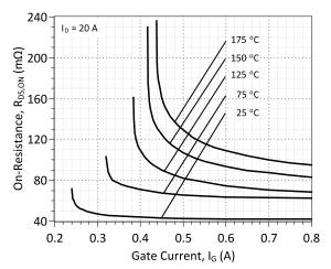
Figure 5: On-Resistance vs. Gate Current
