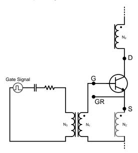
Figure 28: Simplified Current Controlled Proportional Driver
