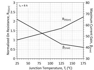
Figure 5: Normalized On-Resistance and Current Gain vs. Temperature
