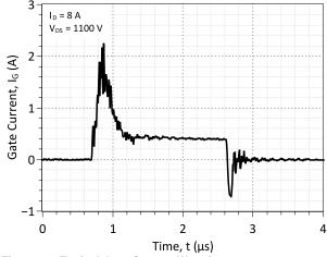
Figure 20: Typical Gate Current Waveform
