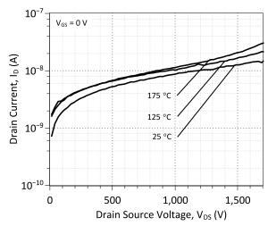
Figure 6: Typical Blocking Characteristics
