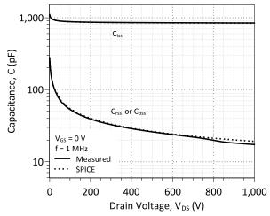
Figure 7: Input, Output, and Reverse Transfer Capacitance
