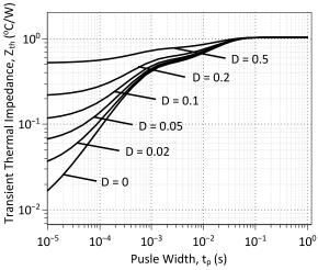
Figure 17: Transient Thermal Impedance
