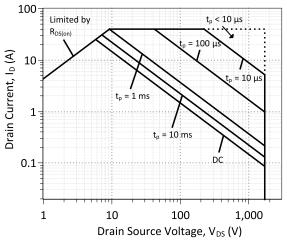
Figure 15: Forward Bias Safe Operating Area at  $T_c$  = 25 °C
