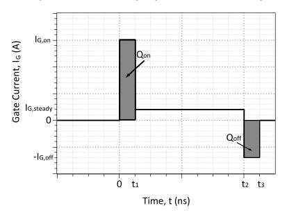
Figure 21: Idealized Gate Current Waveform
