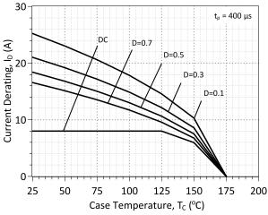
Figure 19: Drain Current Derating vs. Temperature
