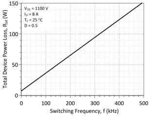
Figure 13: Typical Hard Switched Device Power Loss vs. Switching Frequency <sup>2</sup>
