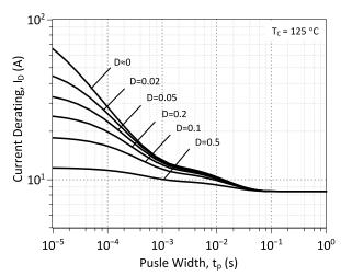
Figure 18: Drain Current Derating vs. Pulse Width
