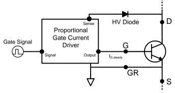
Figure 27: Simplified Voltage Controlled Proportional Driver
