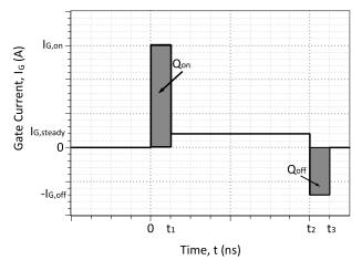
Figure 22: An idealized gate current waveform for fast switching of an SJT.
