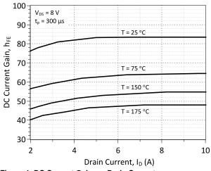
Figure 4: DC Current Gain vs. Drain Current
