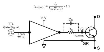
Figure 21: TTL Gate Drive Schematic
