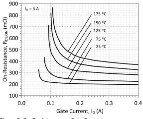
Figure 5: On-Resistance vs. Gate Current
