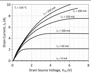
Figure 2: Typical Output Characteristics at 150 °C
