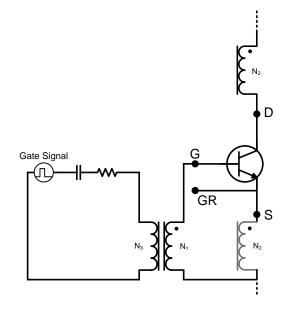
Figure 28: Simplified Current Controlled Proportional Driver
