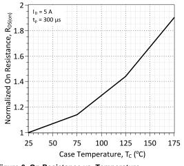
Figure 6: On-Resistance vs. Temperature
