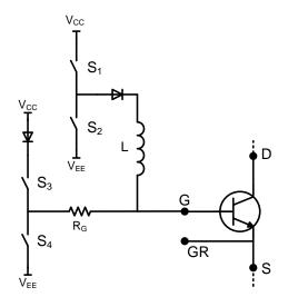
Figure 26: Simplified Inductive Pulsed Drive Topology
