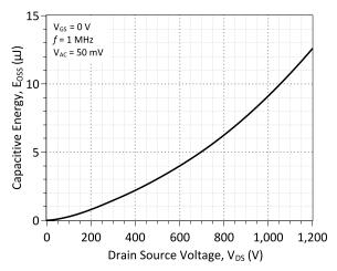
Figure 10: Energy Stored in Output Capacitance
