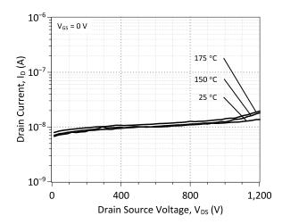
Figure 8: Typical Blocking Characteristics
