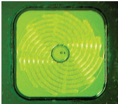
Figure 4: Various Anode-Gate inter-digitations patterns of the Thyristor structure were explored during the development of these Thyristors. An involute pattern shown here was found to provide the best switching performance. In this chip structure, a central Gate terminal provides trigger currents to turn on this Thyristor by flowing the impressed gate current through equidistant Anode-Gate fingers.
