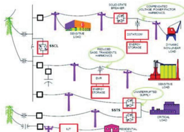
Figure 1: Solid-state current limiters, energy storage elements and solid-state breakers play a critical role in future vision of Smart Grid power electronics based technologies.
