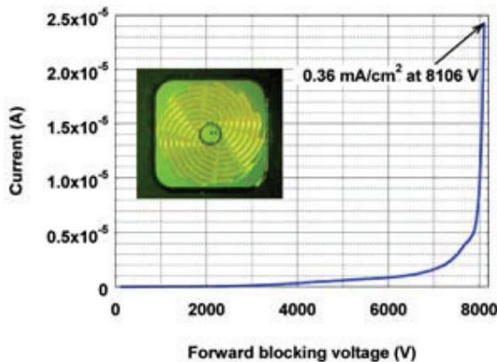
Figure 5a: Forward blocking voltage measured on a representative  $4.1 \times 4.1 \text{ mm}$  involute GTO Thyristor
