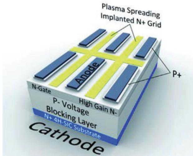
Figure 3: SiC npn Thyristors have their three electrical terminals—Anode and Gate regions on top, and Cathode contact at the bottom. Various SiC layers and their doping types from the top are P+ Anode layer, N-type Gate layer, P- blocking layer, and the N+ Cathode layer. The rated voltage is supported between with n-Gate/p-blocking layers, so that the p-blocking layer doping and thickness primarily determines the breakdown voltage of the device.
