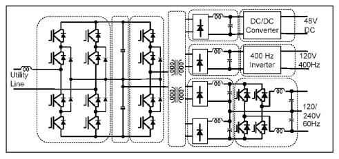
Figure 2. Example three level solid state transformer indicating various secondary output options.
