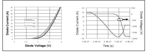
Figure 4. SiC 10 kV PiN diode: (a) current votlage characteristics and (b) reverse recovery characteristics.
